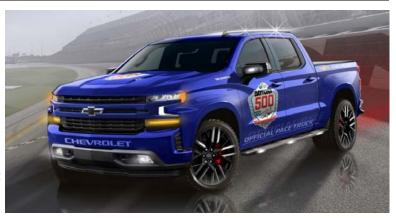
The Silverado pace truck is powered by a production 6.2L V-8 engine paired with a 10-speed automatic transmission. It delivers 420 hp and 460 lb-ft of torque.
